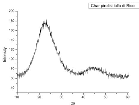
Fig. 2b –XRD pattern of synthesis product obtained at 1500°C
