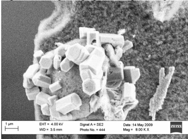
Fig. 3b, SEM photograph of the powder produced at 1600°C – fibers
